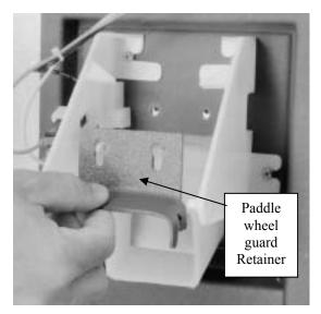
**9** Remove the paddle wheel guard retainer
